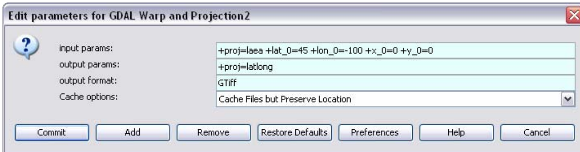
Figure 6.31: The parameters of the GDALWarpAndProjection actor. inputParams and outputParams must be specified in a format used by the GDAL Warp utility.
