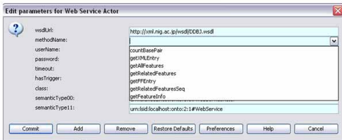
Figure 7.16: The parameters of the Web Service actor. Method names will automatically populate the drop-down menu once a wSDLUrl has been committed.
