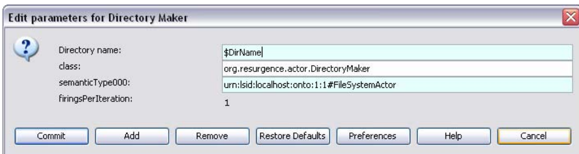
Figure 3.14: Referencing a port-parameter. The $DirName syntax is used to refer to the value of the DirName port-parameter defined on the Workflow canvas.
