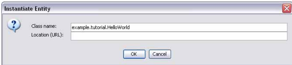
Figure 10.9: To instantiate a new actor, type its class name into the field provided and click OK. The actor will appear on the Workflow canvas.
