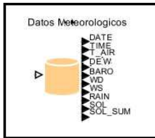
Figure 6.10: An EML 2 Dataset actor customized to output the Datos Meteorologicos data set as fields (the default).
