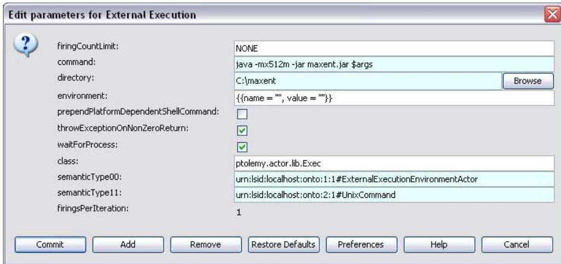
Figure 5.47: The parameters of the ExternalExecution actor.
