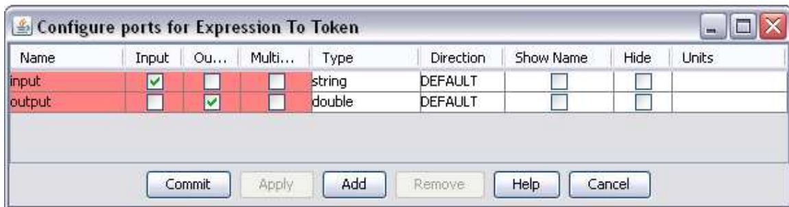
Figure 6.17: Configuring the correct input and output type for the ExpressionToToken actor.
