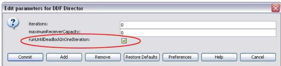
Figure 5.21: Turning on the DDF Director's runUntilDeadlockInOneIteration parameter.
