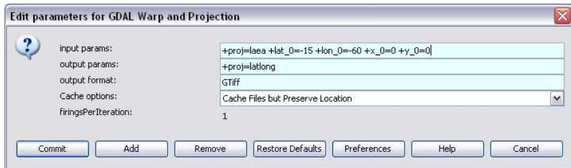
Figure 8.42: The parameters of the GDALWarpAndProjection actor.
