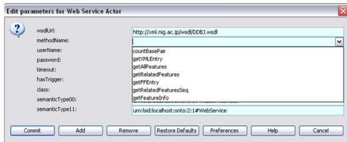
Figure 7.18: The parameters of the Web Service actor. Method names will automatically populate the drop-down menu once a wSDLUrl has been committed.
