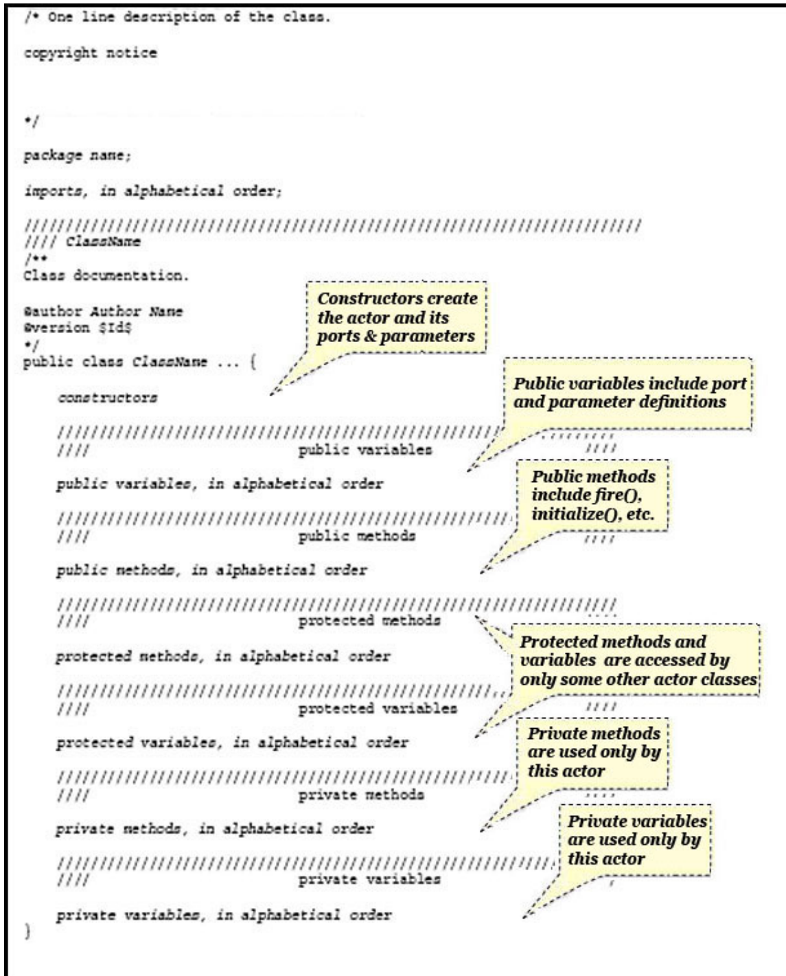
Figure A.2: Generic actor template with major sections identified: constructors, public variables (including ports and parameters), public methods, protected methods, protected variables, private methods, and private variables.
