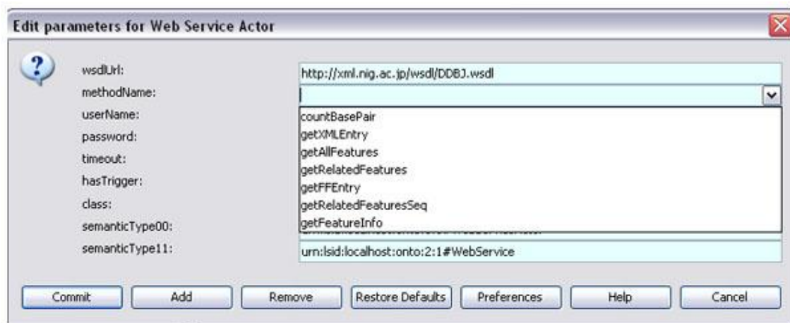
Figure 7.18: The parameters of the Web Service actor. Method names will automatically populate the drop-down menu once a wsdUrl has been committed.
